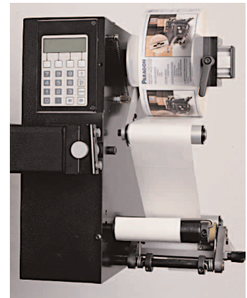
Easy access PLC controls
